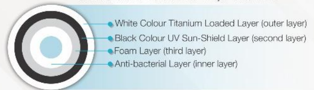
Cross-section of 'Vectus Cool 4 Layer' water tank
