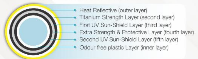
Cross-section of 'Vectus T-90' water tank
