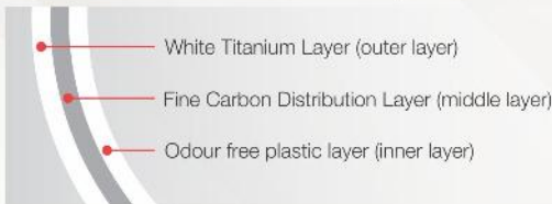
Cross-section of 'Vectus Silk 3 Layer' water tank
