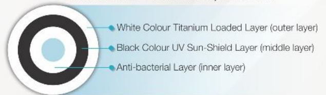
Cross-section of 'Vectus Safe 3 Layer' water tank
