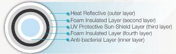
Cross-section of 'Vectus Euro 5 Layer' water tank
