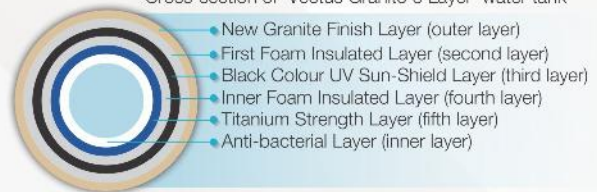
Cross-section of 'Vectus Granito 6 Layer' water tank
