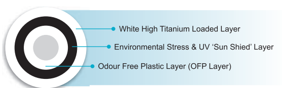
Cross-section of 'Waterwell Pro 3 Layer' Water Tank
