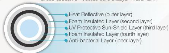
Cross-section of 'Vectus Euro 5 Layer' water tank
