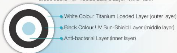
Cross-section of 'Vectus Safe 3 Layer' water tank
