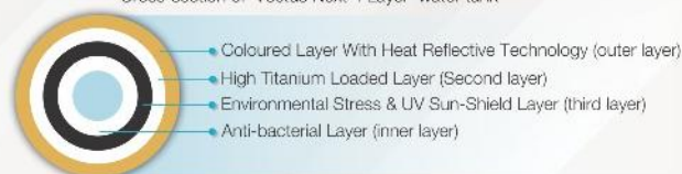
Cross-section of 'Vectus Next 4 Layer' water tank
