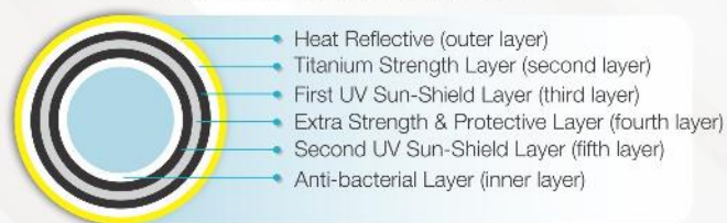
Cross-section of 'Vectus T-90' water tank
