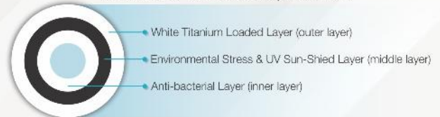
Cross-section of 'Vectus Smart 3 Layer' water tank
