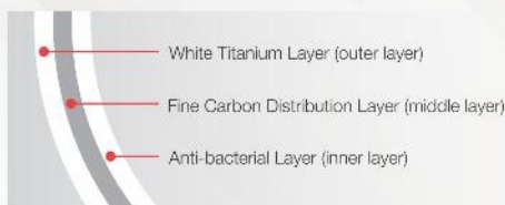
Cross-section of 'Vectus Silk 3 Layer' water tank
