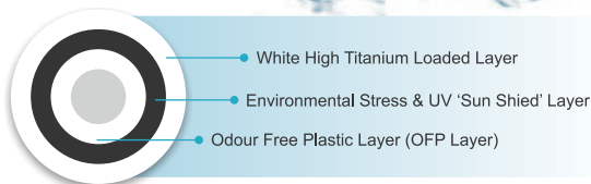
Cross-section of 'Ganga Pro 3 Layer' Water Tank
