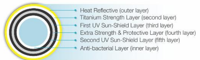
Cross-section of 'Waterwell T-90' water tank
