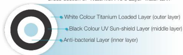
Cross-section of 'Waterwell Pro 3 Layer' water tank
