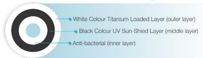
Cross-section of "Waterwell Health 3 Layer" water tank
