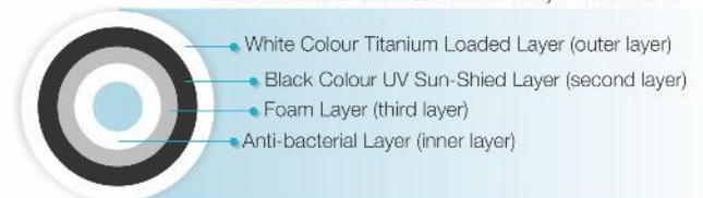
Cross-section of 'Waterwell Italian 4 Layer' water tank
