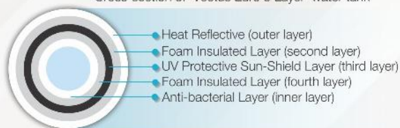
Cross-section of 'Vectus Euro 5 Layer' water tank
