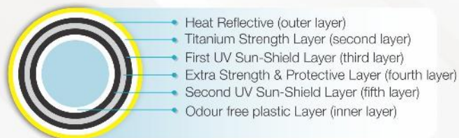
Cross-section of 'Vectus T-90' water tank
