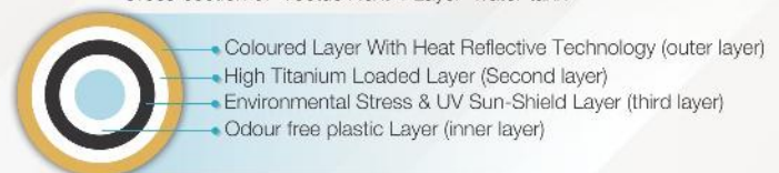
Cross-section of 'Vectus Next 4 Layer' water tank
