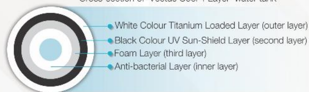
Cross-section of 'Vectus Cool 4 Layer' water tank
