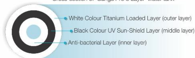
Cross-section of 'Ganga Pro 3 Layer' water tank
