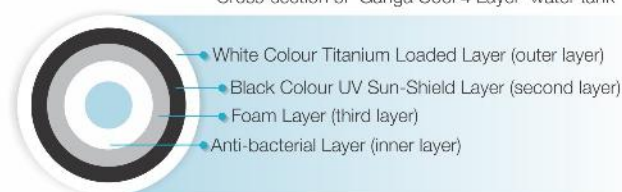
Cross-section of 'Ganga Cool 4 Layer' water tank
