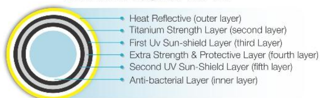
Cross-section of 'Ganga T-90' Water tank
