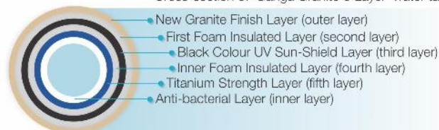
Cross-section of 'Ganga Granito 6 Layer' water tank
