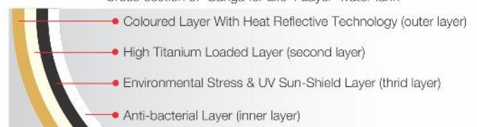
Cross-section of 'Ganga for Life 4 Layer' water tank
