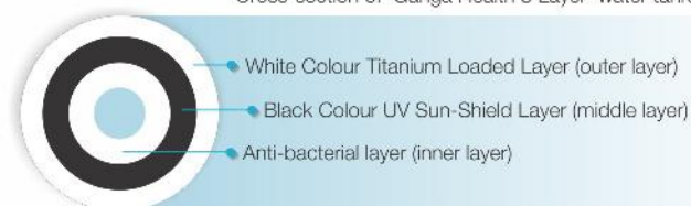
Cross-section of 'Ganga Health 3 Layer' water tank
